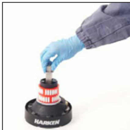
8. Slide out the central shaft n°19
