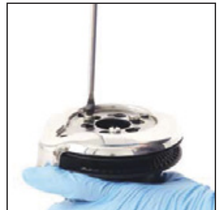
6. Unscrew the three screws n°27 (4 Nm/35 in-lb)
