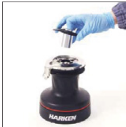
5. Slide off the hub n°28 and the cover n°29
