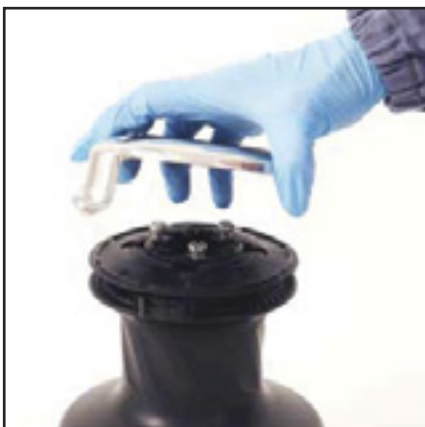
7. Remove the self-tailing arm n°26 by rotating and lifting it.
