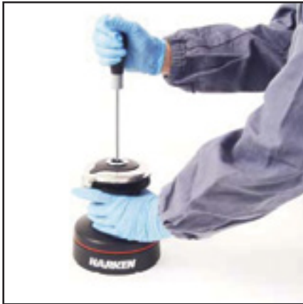
1. Unscrew the central screw (2 Nm/18 in-lb)
