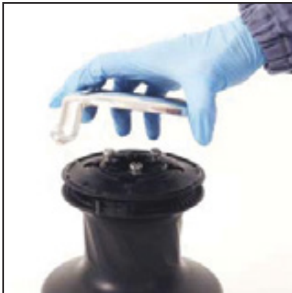
4. Remove the self-tailing arm n°26 by rotating and lifting it.
