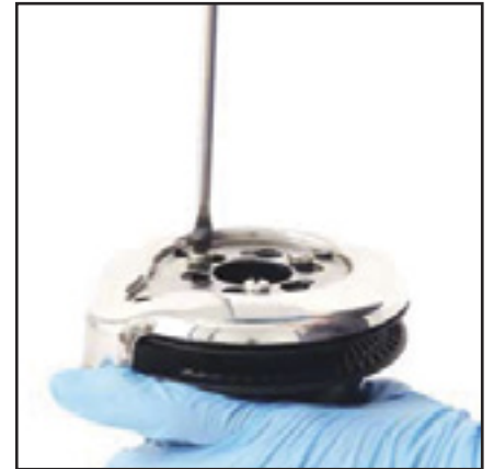
3. Unscrew the three screws n°27 (4 Nm/35 in-lb)
