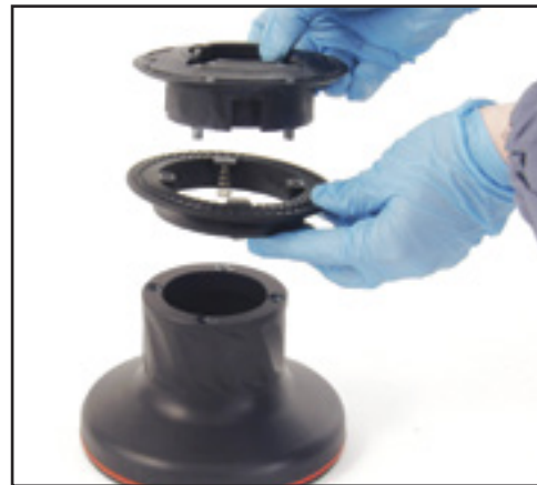
If jaws have been disassembled, insert peeler between two jaws, taking care that letters "TOP" on peeler are facing upwards.
