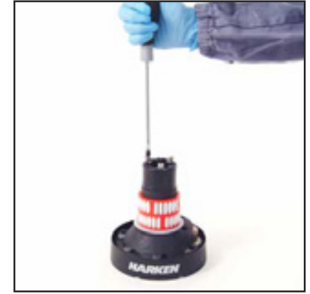
6. Completely unscrew three screws n°27
