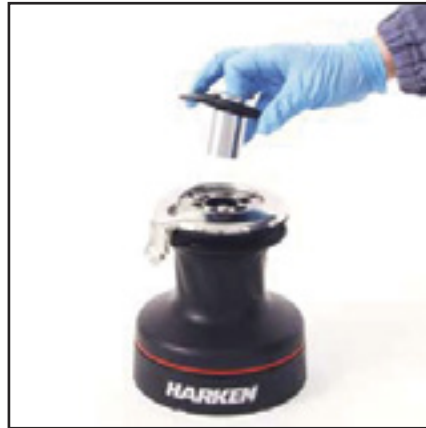
2. Slide off the hub n°28 and the cover n°29
