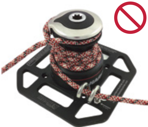
Excessive turns at base of winch
