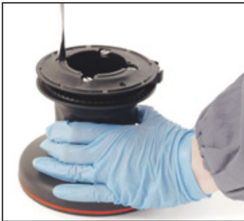
When positioning stripper arm, align peeler with it.
