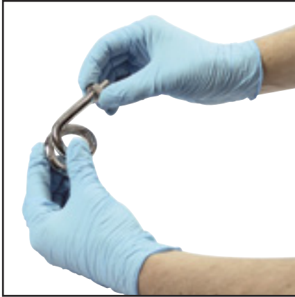
1. Install nut on pigtail. NOTE. Pigtail should be installed with no thread locker.
