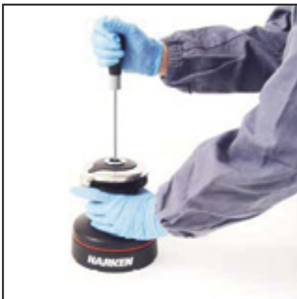
4. Remove winch handle socket.
