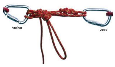
To release the radium release hitch, untie the overhand-on-abight that secures the hitch. Maintaining tension on the Münter hitch, carefully untie the half hitch below the Münter hitch. Slowly feed line through the Münter hitch to allow the radium hitch to lengthen and lower the load. When the load has been transferred to the main line, re-secure the radium release hitch by tying a half hitch and an overhand-on-a-bight below the Münter hitch.
