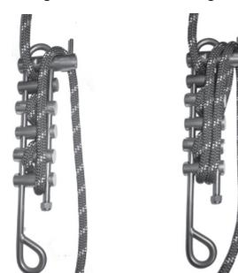
Repeat action for a second loop and tie off a bite of rope crosswise around the rack for final security of the rope. Fig. E, F & G.
