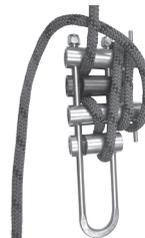
**Step 2:** Bring the tail end of the rope around the leading end of the rope (where the leading end contacts the first Tie-Off Bar).
