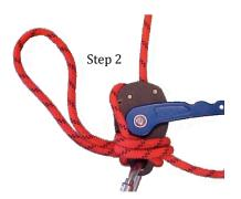
Finish with an overhand knot so that the bite of the rope is pointing towards the attachment point of the device.
