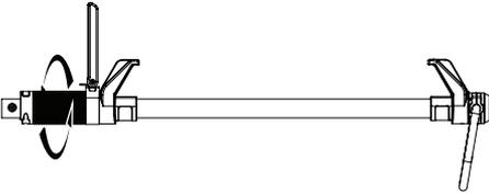
2. Fully loosen nut by turning counterclockwise.
