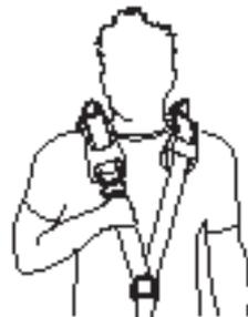
Fasten upper harness section to lower harness section using the AustriAlpin COBRA™ Quick Connect Buckle on the shoulder.
