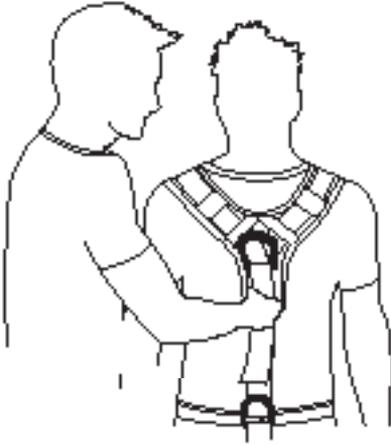
Have a partner adjust the back adjustment strap that is attached to the dorsal D-ring until the dorsal D-ring is positioned between the shoulder blades. Once this adjustment is made, it should not need to be changed if the same person is using the harness subsequently.
